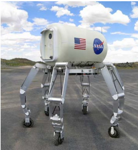
NASA's All-Terrain Hex-Limbed Extra-Terrestrial Explorer (ATHLETE) rover is being developed by JPL as part of JSC's Human Robotics Systems Project.
