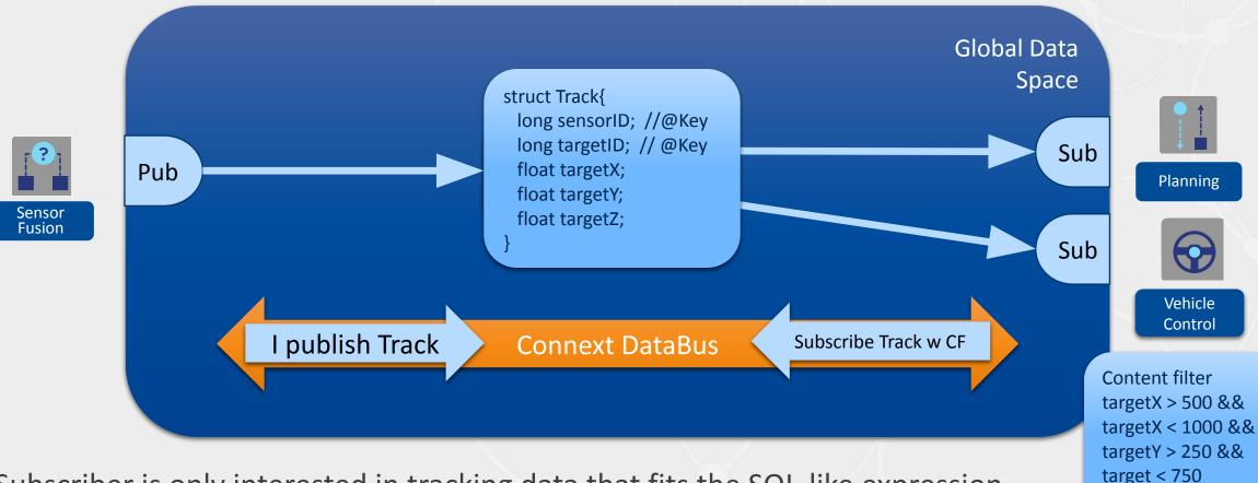
Subscriber is only interested in tracking data that fits the SQL-like expression above(Content Filter). The Content Filter itself is propagated to the publisher. If no one is interested in a particular sample based on that filter, that packet is NOT transmitted (vs sent and ignored by subscriber).
