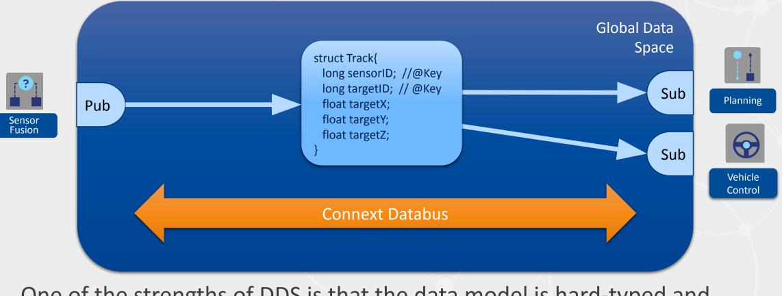
One of the strengths of DDS is that the data model is hard-typed and shared. This means DDS can apply intelligence to messages since it can understand the contents. This is what we call data-centricity.
