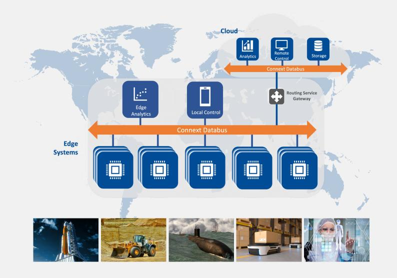
Connext Anywhere solves this challenge with RTI Cloud Discovery Service, which enables dynamic discovery between applications on private networks. Applications can establish peer-to-peer communication across networks without multicast and with support for NAT traversal from private to public, as well as from private to private addresses, the latter with the help of Cloud Discovery Service running in the cloud (or anywhere publicly visible).
