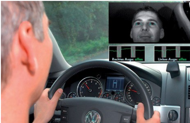
Figure 9. Volkswagen's driver assistance and integrated safety system uses Connex DDS to combine radars, laser range finders and video to assist safe operation. It tracks the driver's eyes to detect drowsiness. It also detects lane departures, avoids collisions and helps keep the car in its lane.
