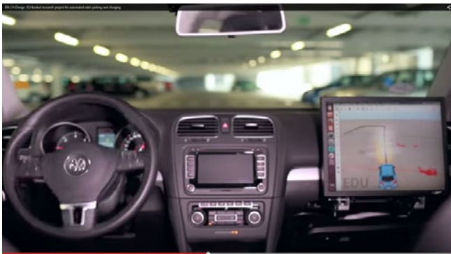
Figure 10. The V-Charge program, executed by VW, Bosch and ETH Zurich, implements an electric vehicle that can drop off its passenger, then drive autonomously to a parking lot, park itself and take its turn at a charging station. The system was successfully demonstrated in 2014.
