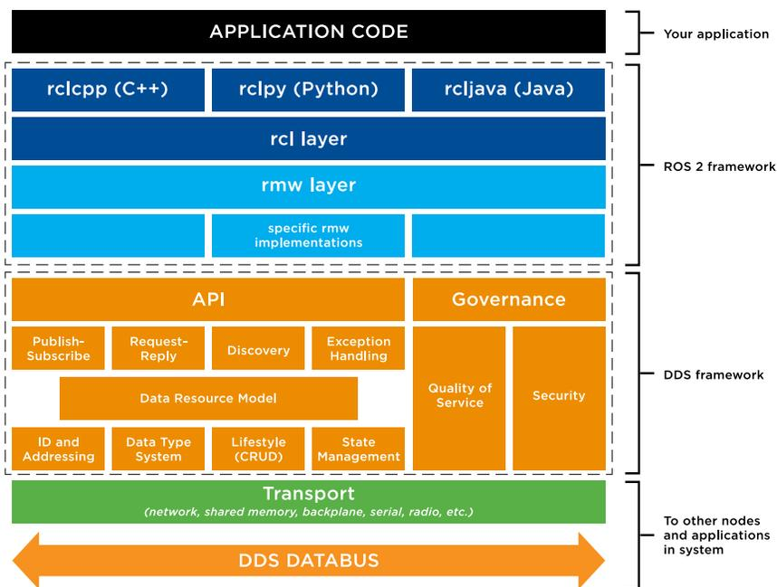
Figure 1: Illustration of DDS/ROS 2 technology stack
