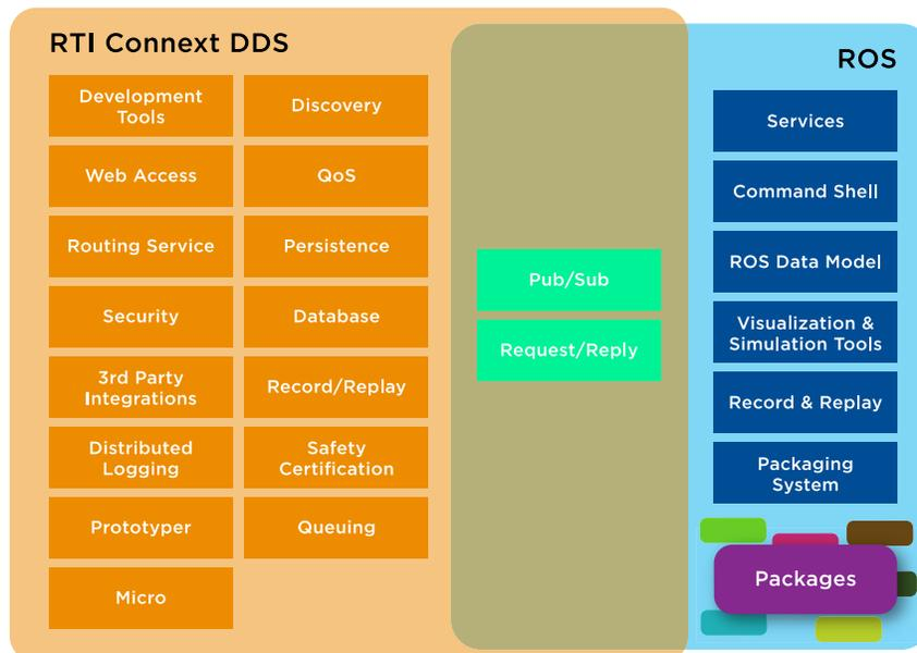
Figure 4: Intersection of RTI Connex and ROS functionality
