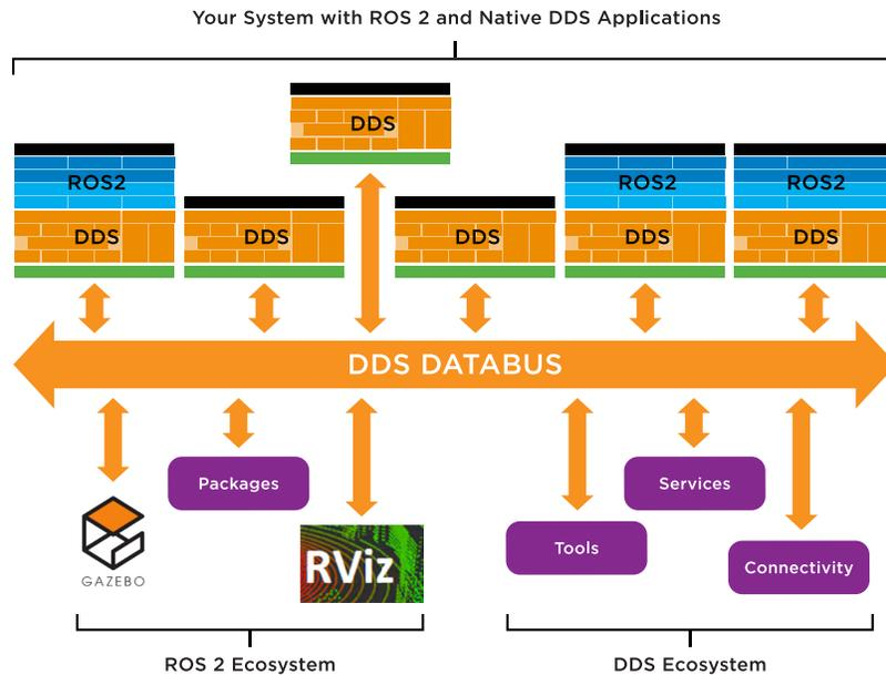
Figure 3: DDS and ROS 2 hybrid system and ecosystem
