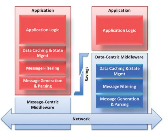
Figure 1: Illustrates the differences between message-centric and data-centric approaches with respect to consumer-side logic
