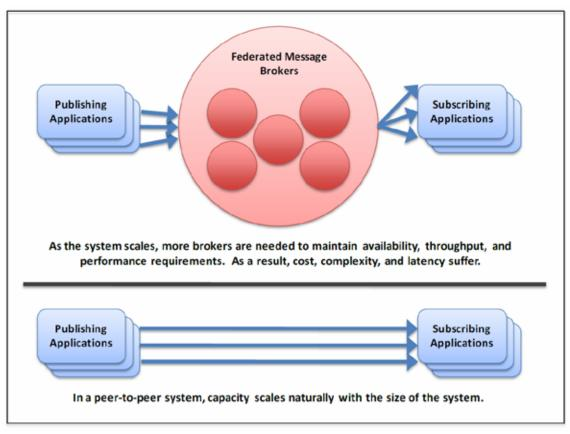
Figure 3: Peer-to-peer architectures are far more scalable than broker-based systems
